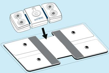
2. Clip the 4 cables onto the lumbar electrode and on the actiTENS
